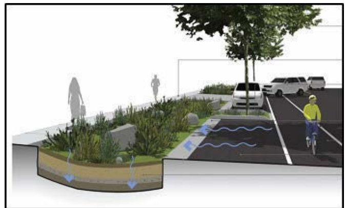
Street runoff flowing into vegetated areas that capture and treat polluted stormwater (Image courtesy of Callander Associates and the City of Campbell)
